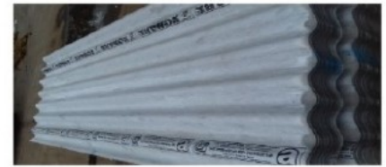
Fiber Cement sheet
